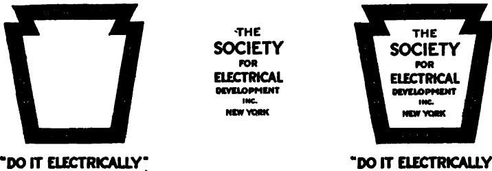
Fig. 116. — Illustrating a flashing sign produced by properly relating the hue and brightness of the pigments with the colors of the illuminant.
